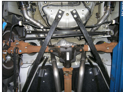
Photo 2- Over-axle pipe routing
