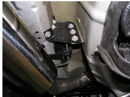
Photo 4- left muffler rear hanger bracket installed
