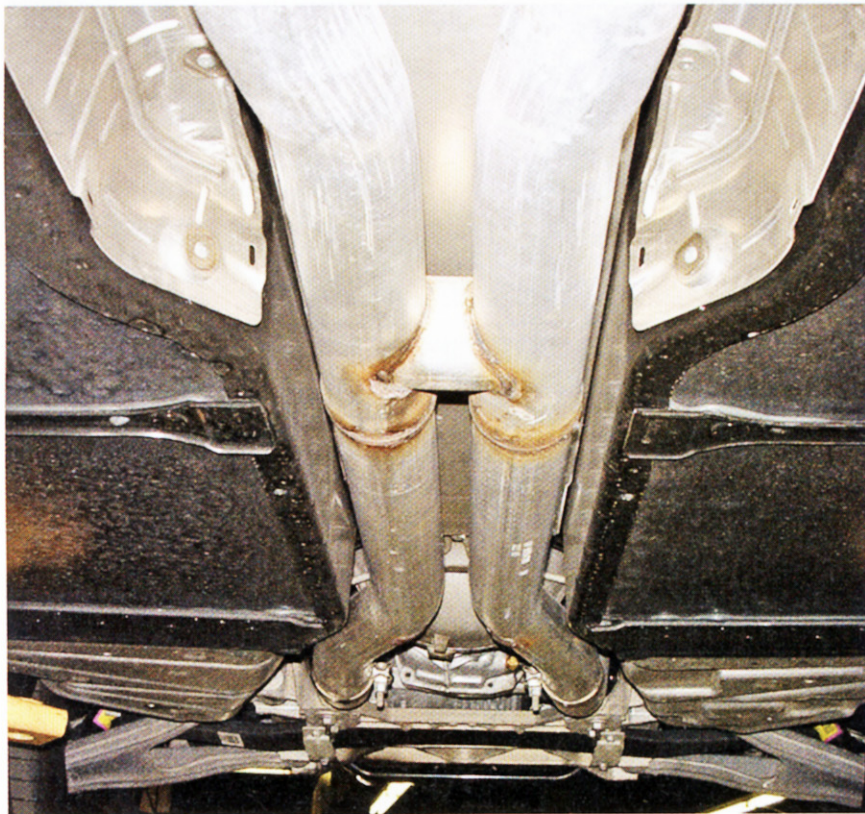
Like all new Zs, ours came from the factory with a traditional H-pipe...
