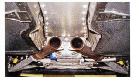
The Bassani system installs here, just behind the catalytic converters. Since all factory smog equipment is retained, vehicle emissions should be unaffected.
